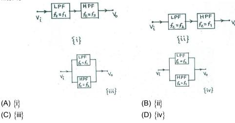
18. Refer to the schematic diagram in Q. No. (47). The combination that works as a band elimination filter is
