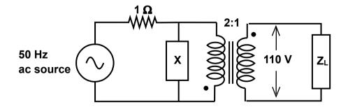
Assuming the transformer to be ideal, the value of the reactance X to improve the input power factor to unity is \_\_\_\_\_\_.
