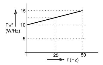
The hysteresis and eddy current losses of the transformer at 25 Hz respectively are
