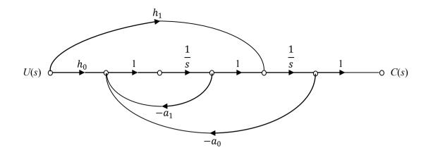
Assuming,  $h_1 = b_1$  and  $h_0 = b_0 - b_1 a_1$ , the input-output transfer function,  $G(s) = \frac{C(s)}{U(s)}$ of the system is given by
